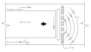
Figure 2. Single U-shaped ventilation air flow direction
