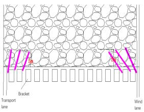
Figure 1. Schematic diagram of corner cannula grouting
