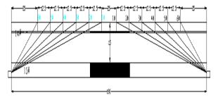
Figure 3. Fan-shaped water spray hole arrangement
