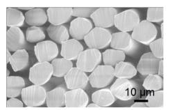
Figure 1: Cross-sectional SEM image of the nano silver antibacterial polyester fibers.
