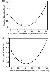
Figure 3: Breaking strength (a) and elongation at break (b) for the nano silver antibacterial polyester combed cotton yarn.
