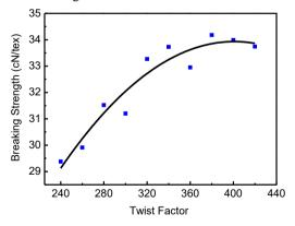
Figure 4: Influence of twist factor on the nano silver antibacterial terylene pure yarn breaking strength.
