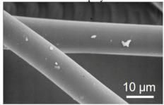
Figure 2: Longitudinal section SEM image of the nano silver antibacterial polyester fibers.
