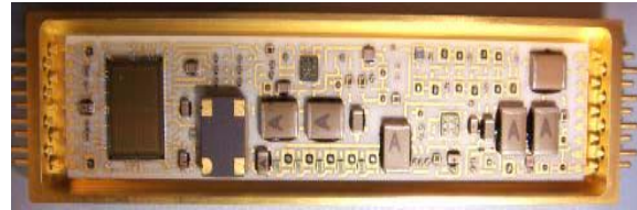
Figure 2 .Permanent Down-hole Gauge
