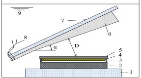
Fig.4 The method of regulated underwater shockwave 1 foundation, 2 base plate, 3 gap, 4 flyer plate, 5 cover plate, 6 explosive, 7 reflection thick plate, 8 detonation, 9 water
